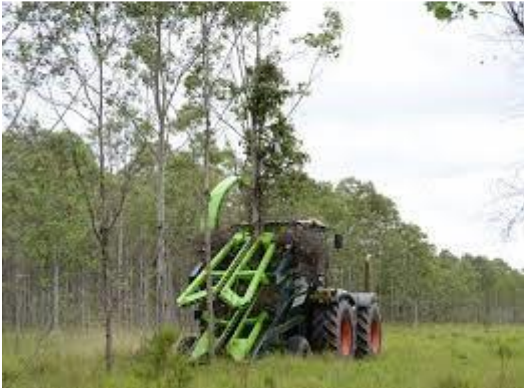
Figure 5-14 Bionic Beaver prototype harvesting larger single stem trees
