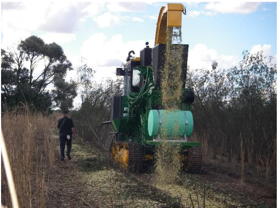
Figure 5-12 2009 Model Canetec Leucaena Harvester in operation
