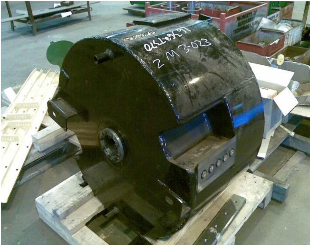
Figure 5-11 Main drum 2009 Leucaena Harvester build
