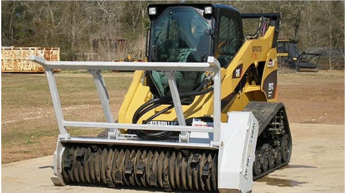
Figure B-2 Commercial mulching attachment (75HP range) – trees to 250 mm diameter
